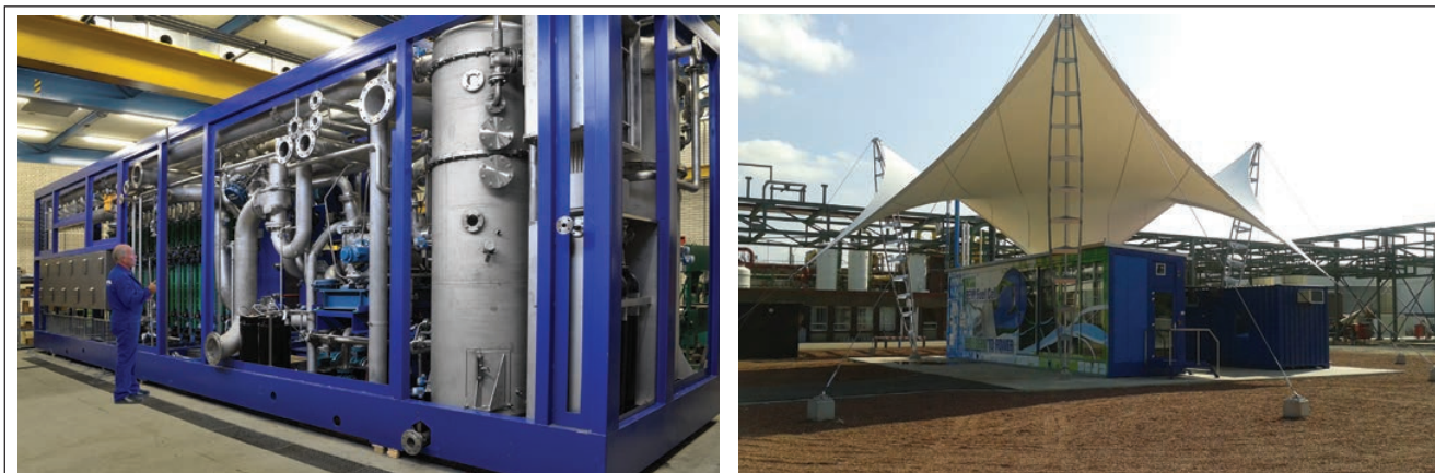
Nedstack's 1 MW PEM Power Plant has been in operation with Solvay in Lillo, Belgium since early 2012.
